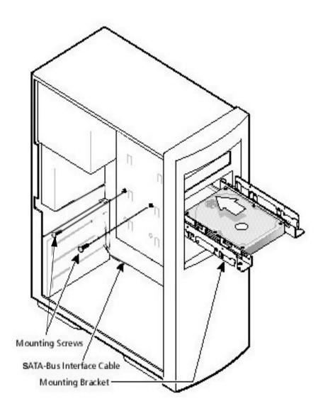
Figure 4-8 Completing the Drive Installation
