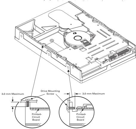
Figure 4-5 Mounting Screw Clearance
