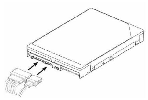
Figure 4-7 Drive Power Supply and SATA Bus Interface Cables
